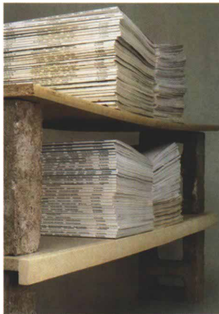
Aprons stiffen the shelves. Putting a solid-wood apron on a shelf increases its load-carrying capacity. The sagging top shelf is ¾-in. particleboard. The virtually straight bottom shelf is ¾-in. particleboard with a 1x2 apron glued to the front edge.
