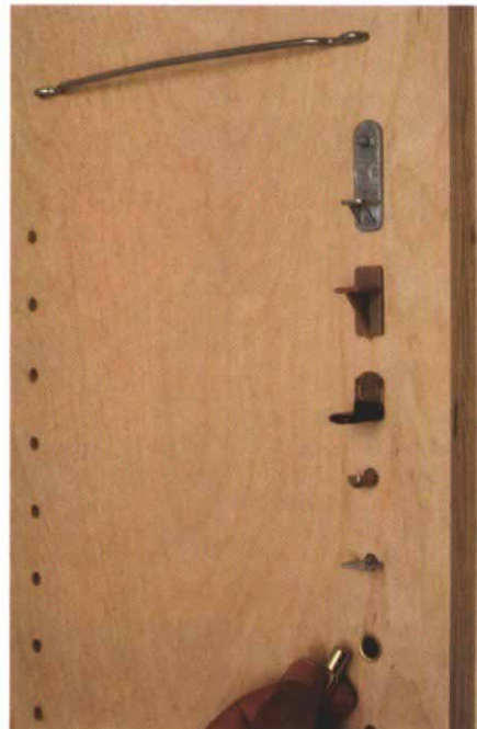
Shelf pins are inconspicuous. Shelf pins are less visible than shelf standards. Top to bottom: wire clip, which hides inside a groove at the end of a shelf; spring-loaded locking clip that prevents shelves from sliding or tipping; plastic cushioned metal L-support; zinc-plated steel paddle; "library" pin with sleeve.
