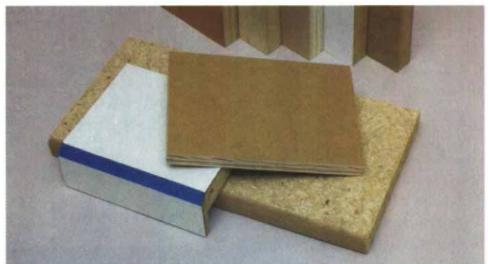
Sheet stock is a stable and uniform choice for shelving. Options range from hardwood-veneer plywood to medium-density fiberboard panels with a durable melamine surface.
